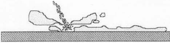
FIGURE 3. CO 2 gas expansion and pellet kinetic effects break away and remove coating particles.
